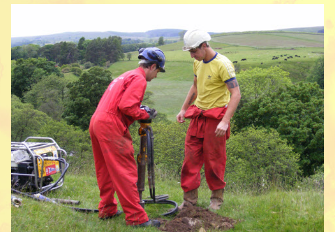
2009 boreholes sunk on two cross-sections of north slope and movement monitoring points installed
